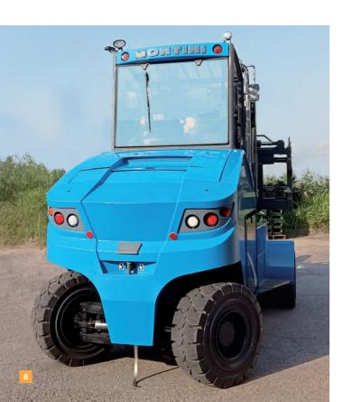
Every technical aspect has been designed to make forklift operation easy in any working situation: from the **unique sloping of the counterweight**, which guarantees perfect visibility when reversing, to the **large grab handle**, for getting into the operator's seat with ease.
