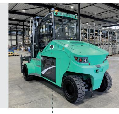
The **battery is charged in direct mode**, using the easily accessible connector protected by a convenient cover flap, as with electric cars.
