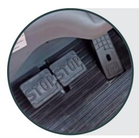
A large, spacious pedal board with **single drive pedal** (with forward/reverse switch button on the provided hydraulic control armrest) combined with a large brake pedal.
