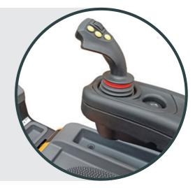
The simple to use and easily accessible **hydraulic control with fingertips** (mini-levers) is installed in an ergonomic and adjustable armrest.
