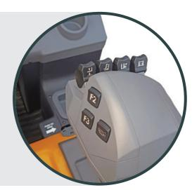
The **hydraulic control with pilot levers** (minijoysticks) makes driving the forklift truck easy and reliable. Easily accessible and simple to use, it is installed in an ergonomic, adjustable armrest to guarantee comfortable driving positions.
