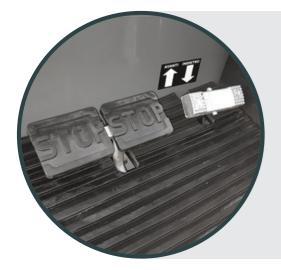
Pedal board with a **rocker-type forward/reverse pedal** and a wide, comfortable brake pedal, to assure a safe and secure foothold.
